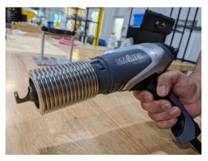
1. This instruction is to install an Insulon Safety Guard onto a Steinel HG 2320 E heat gun with a 14mm reflector nozzle.
