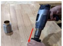
2. Remove the black plastic cover by rotating it counter-clockwise and separating it from the heat gun.
