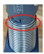
3. Place the Safety Guard on a flat surface and insert heat gun nozzle into the Insulon safety guard.
