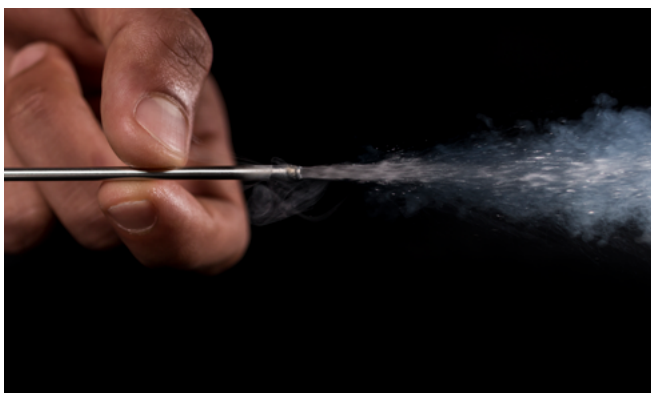
Figure 1: Liquid nitrogen ( -196^{\circ}\text{C} ) flows through an 11 gauge Insulon® Sheath. The external surface remains near ambient temperature allowing for safe contact with healthy tissue.
