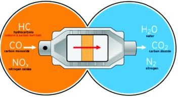
*Figure 2:* Harmful engine emissions enter the catalytic converter and exit as water vapor, nitrogen and carbon dioxide<sup>[4]</sup>.
