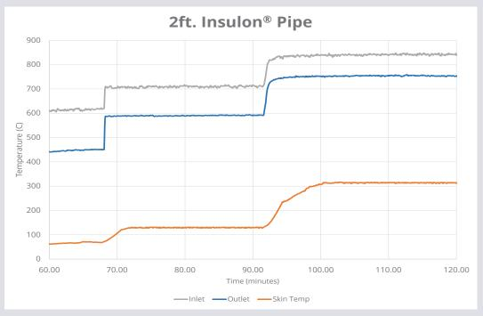
*Figure 4:* Insulon® case study showing temperature drop across two foot tube wrapped with Insulon and the skin temperature mid-length of the tube on the outer surface.
